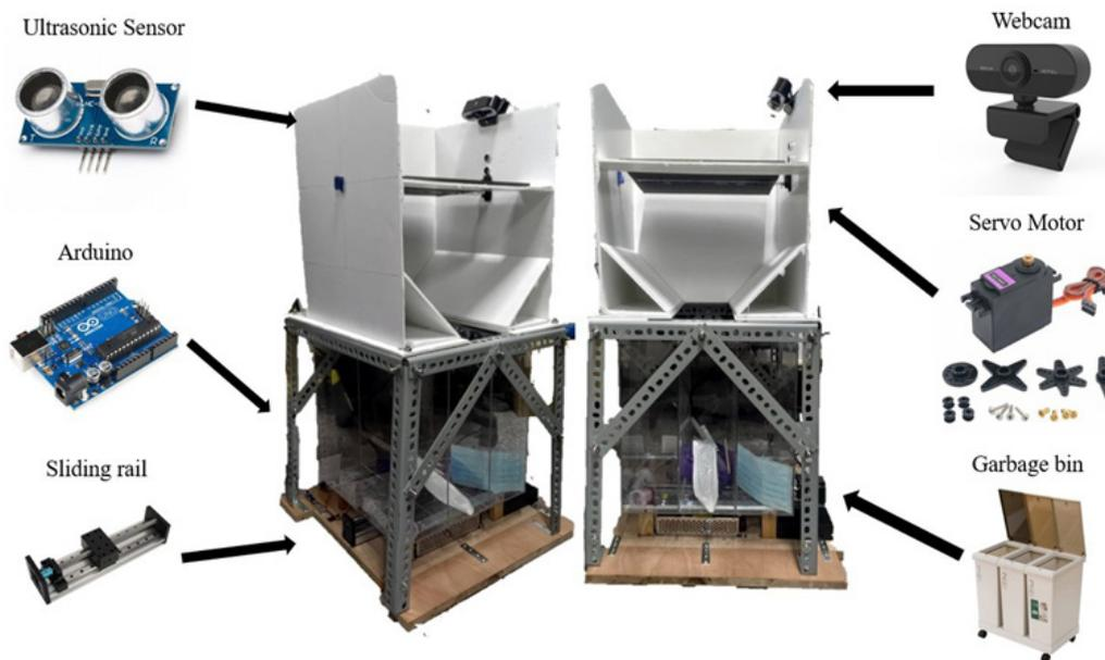
Figure 5. The hardware setup of the automatic medical waste classification mechanism
