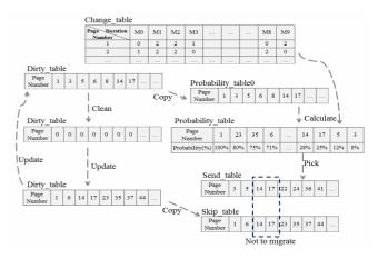
Figure 4. The flowchart of predicted method [18]
