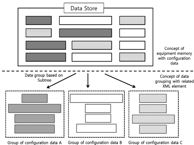
Figure 3. Concept of the <partial-lock> operation for the partial locking of the data store and grouping based on their interdependency
