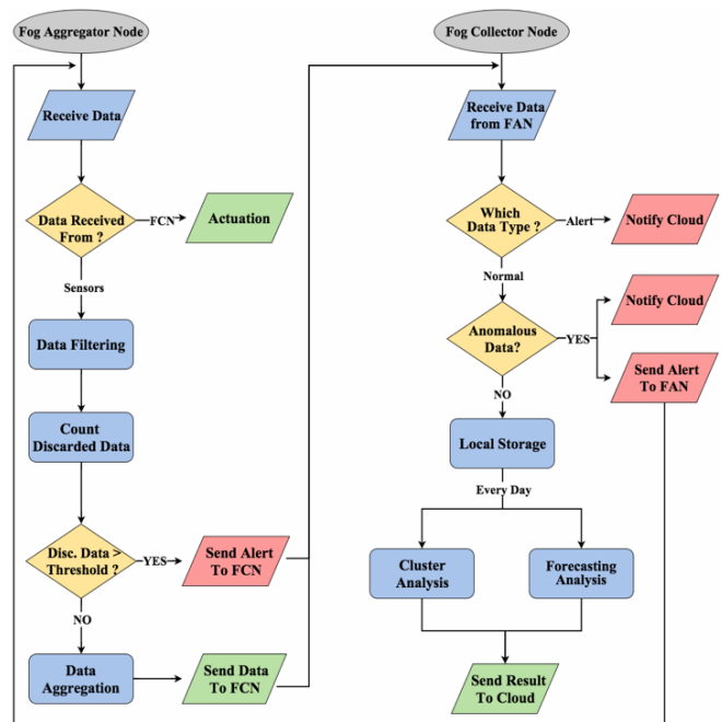
Figure 4. Flow diagram which describes the Fog logic
