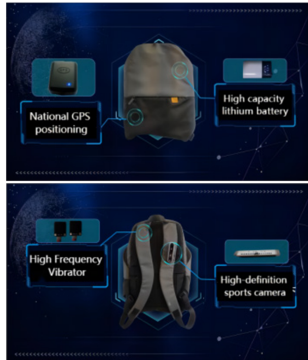
Figure 1. Structure diagram of the smart assistive blind backpack
