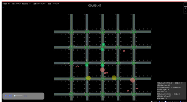
Figure 11. Simulation example of priority control for emergency rescue vehicles
