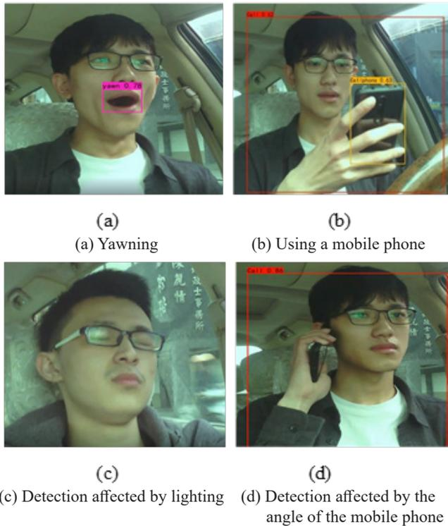
Figure 7. Actual in-vehicle state detection results
