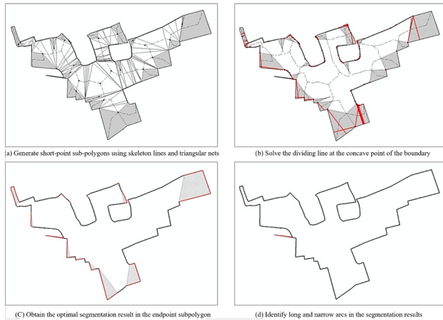
Figure 4. Recognition of long and narrow arcs by skeleton based decomposition
