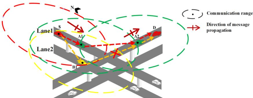
Figure 2. The two-hop connection probability reduction in 3D scenario
