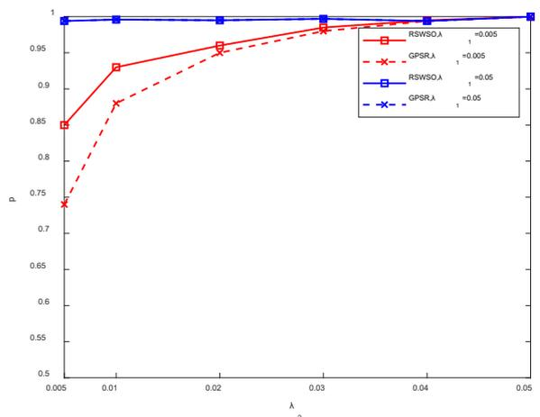
Figure 6. The two-hop connection probability versus node density
