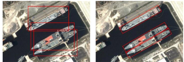
Figure 1. Comparison of HBBs and OBBs. For adjacent ships, HBBs in image (a) have a larger overlap area than OBBs in image (b), and boxes with lower confidence scores will be suppressed.
