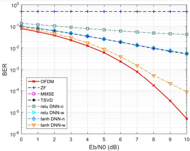
Figure 7. BER versus  $E_b/N_0$ ,  $\alpha = 0.9$ , QPSK modulation
