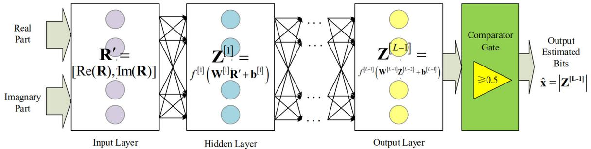
**Figure 3.** The implementation of the block of Information Bits Recovery
