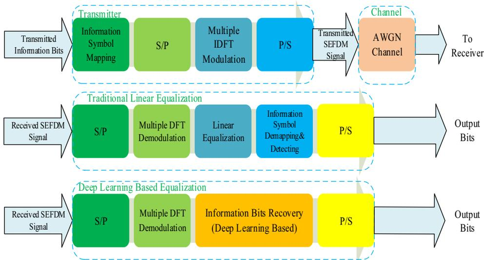
**Figure 1.** SEFDM system model based on linear equalization and DL-based equalization scheme
