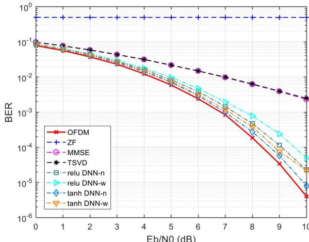
Figure 5. BER versus  $E_b/N_0$ ,  $\alpha = 0.8$ , BPSK modulation
