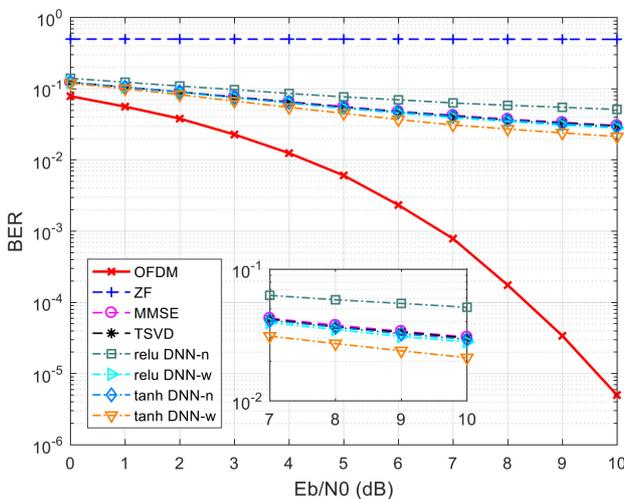
Figure 8. BER versus  $E_b/N_0$ ,  $\alpha = 0.8$ , QPSK modulation
