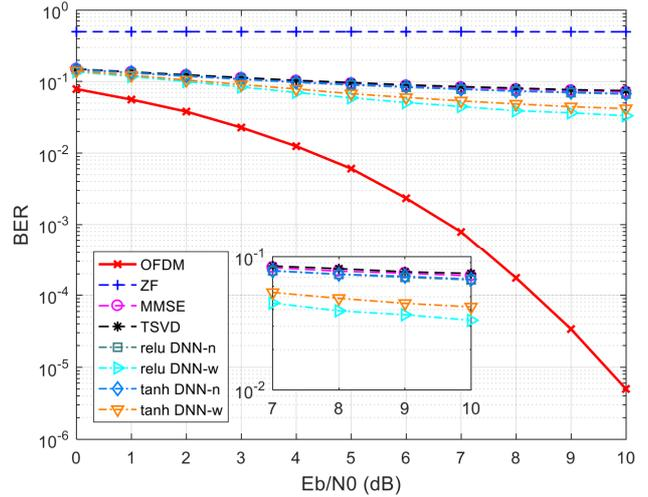
Figure 9. BER versus  $E_b/N_0$ ,  $\alpha = 0.7$ , QPSK modulation
