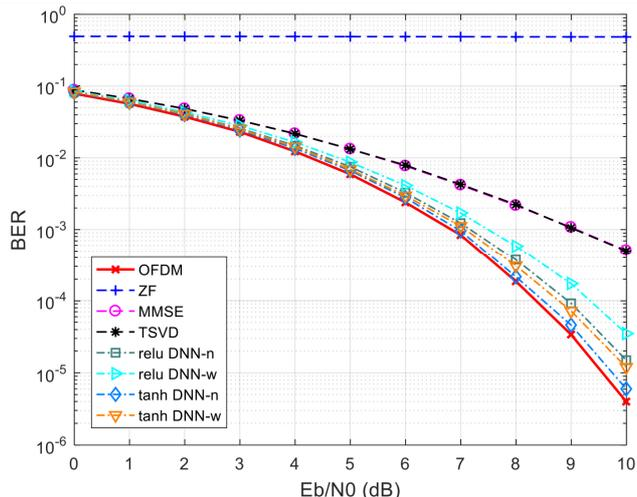
Figure 4. BER versus  $E_b/N_0$ ,  $\alpha = 0.9$ , BPSK modulation
