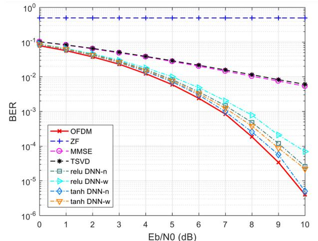
Figure 6. BER versus  $E_b/N_0$ ,  $\alpha = 0.7$ , BPSK modulation
