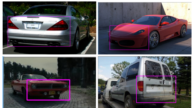
Figure 7. Results of vehicle detection when shadows were casted on the analyzed vehicles
