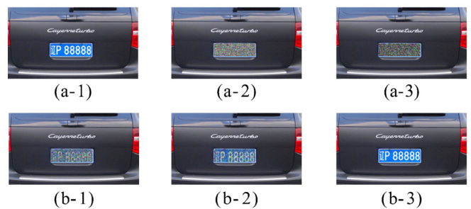
Figure 6. Simulation results of regional progressively recovery on a color image ‘Car’ with ((1, 3), 3, 3, 6) threshold
