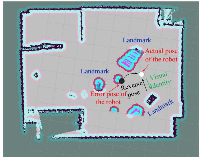
**Figure 9.** The process of correcting the pose by using the landmark
