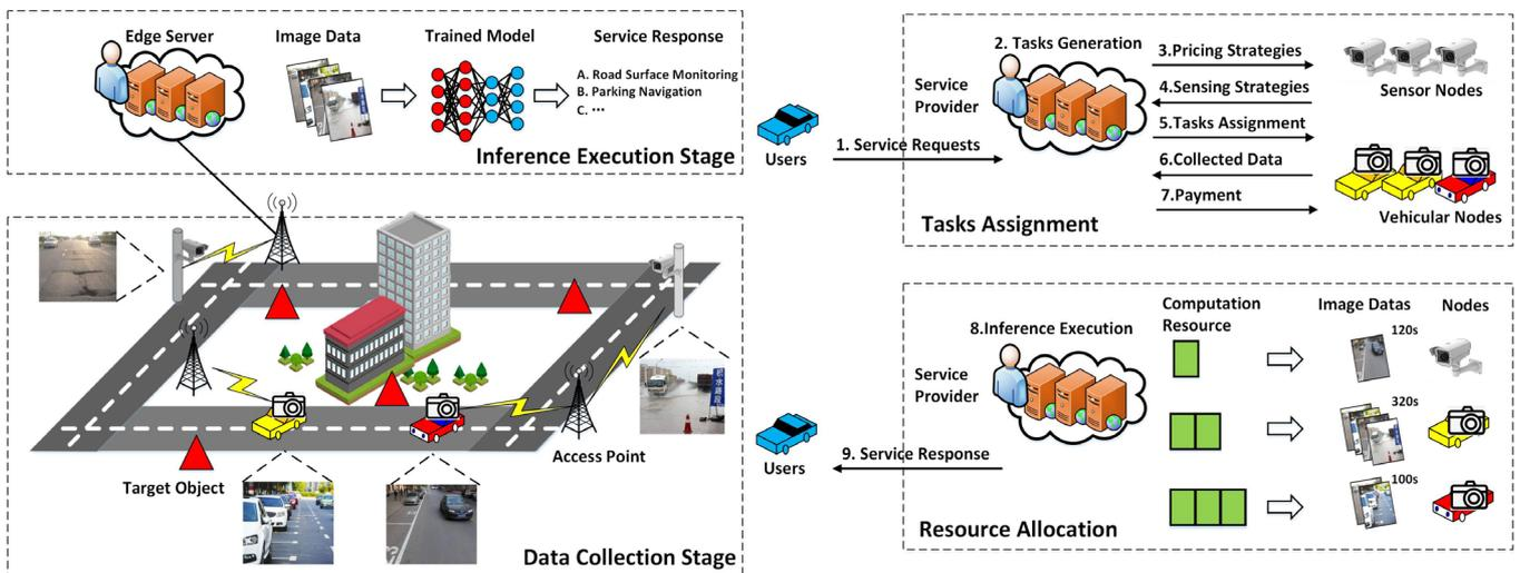
**Figure 1.** The system integrating hybrid sensor network and edge computing for AI applications of connected vehicles
