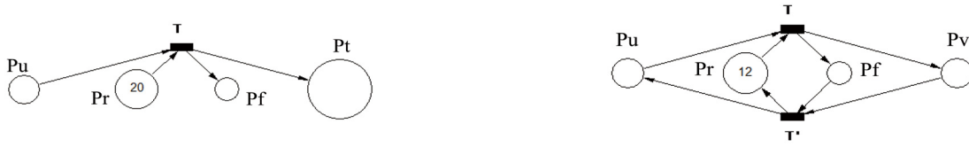
(a) An instance for Algorithm 3 running from step 7 to 13 for (u,v) \in E \wedge v=t , where forward Place P_f and revise Place P_r with a specified number of tokens are added into the model
