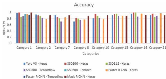
Figure 10. Performance comparison between the algorithms and frameworks on each categories in terms of accuracy
