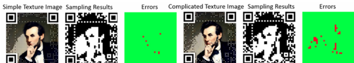
Figure 1. Error analysis of the intermediate results of scanning different QR codes using the ZXing library
