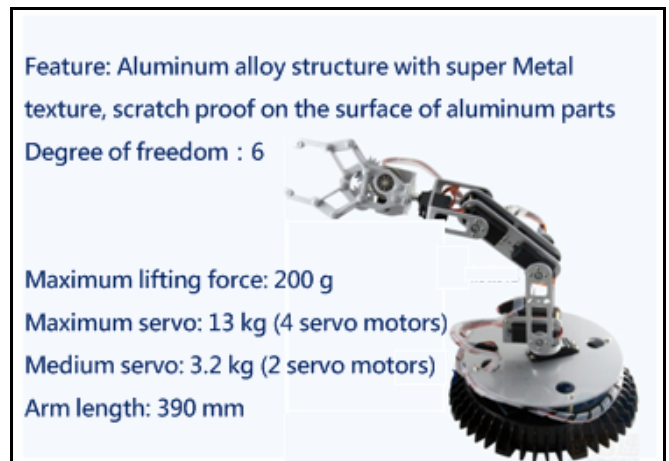
Figure 7. Specifications of the six-axis robotic arm
