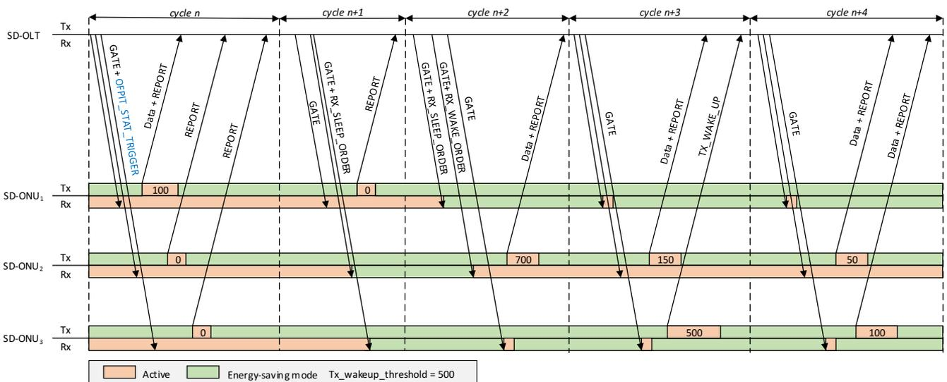
Figure 3. Proposed SD-ONU energy-saving operation
