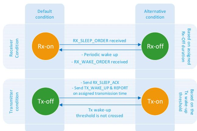
(b) Proposed ONU transmitter and receiver conditions
