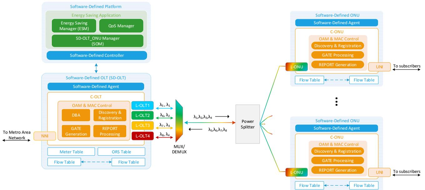
**Figure 1.** Proposed software-defined TWDM-PON energy-efficient architecture
