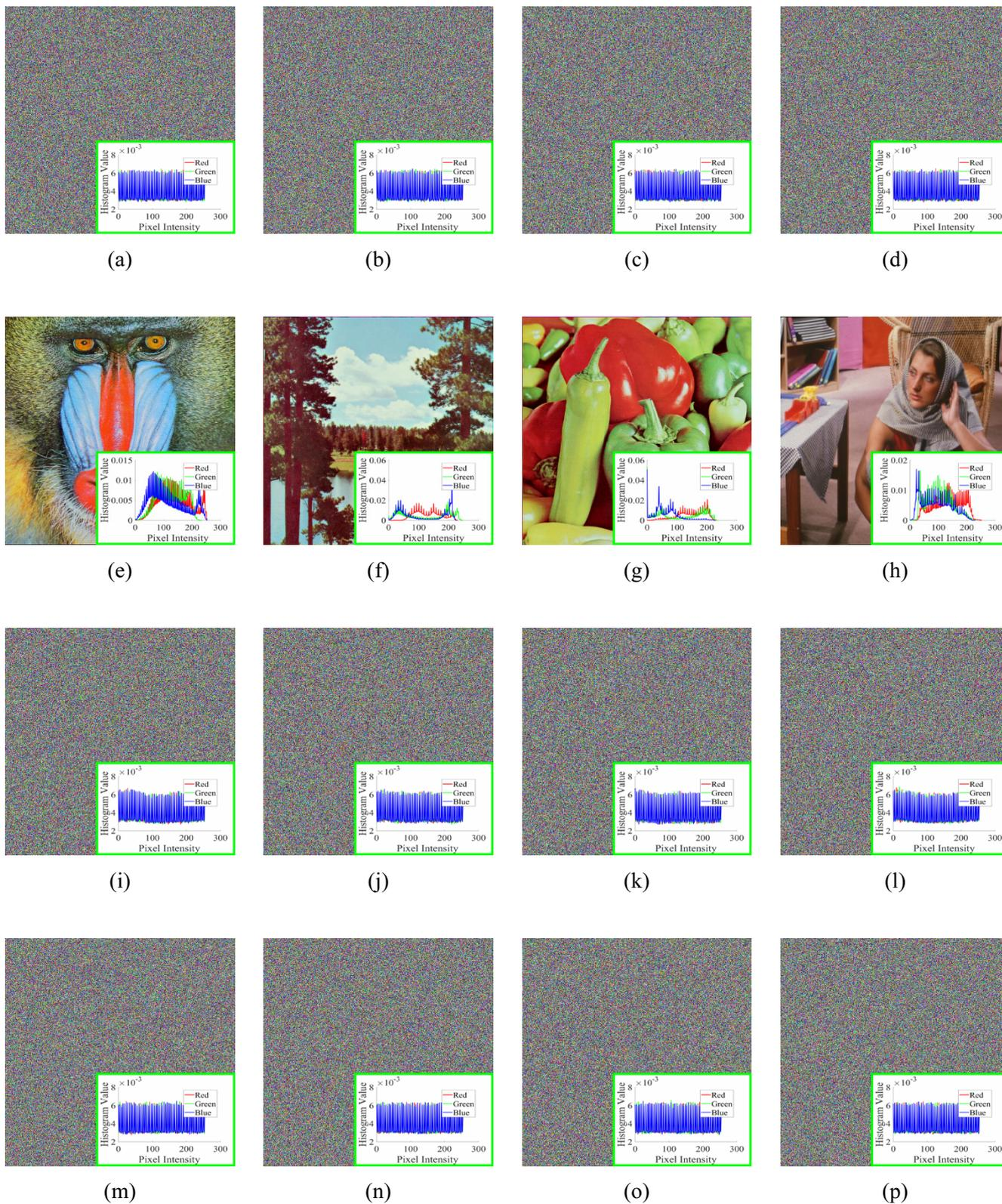
**Figure 4.** Proposed method with random image, for  $n = 4$  : (a)-(d)  $\{S_1, S_2, S_3, S_4\}$  . (e)-(h)  $\{I_1, I_2, I_3, I_4\}$  recovered with correct chaotic keys. (i)-(l)  $\{I_1, I_2, I_3, I_4\}$  recovered with incorrect chaotic keys. (m)-(n)  $\{I_1, I_2\}$  recovered from  $n - 1$  shared images. (o)-(p)  $\{I_1, I_2\}$  recovered from  $n-2$  shared images.
