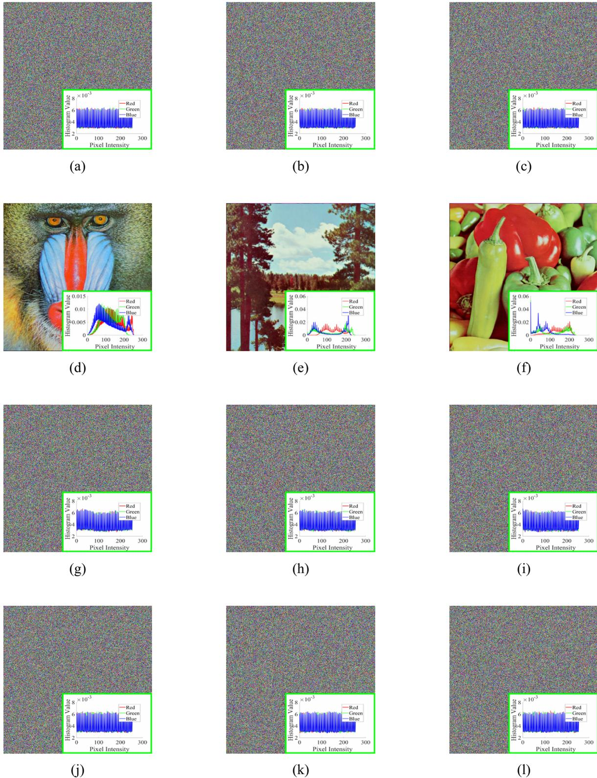
**Figure 5.** Proposed method with random image, for  $n=3$ : (a)-(c)  $\{S_1, S_2, S_3\}$ . (d)-(f)  $\{I_1, I_2, I_3\}$  reconstructed with correct chaotic keys. (g)-(i)  $\{I_1, I_2, I_3\}$  reconstructed with incorrect chaotic keys. (j)-(k)  $\{I_1, I_2\}$  reconstructed from  $n-1$  shared images. (l)  $\tilde{I}_1$  reconstructed from  $n-2$  shared images.
