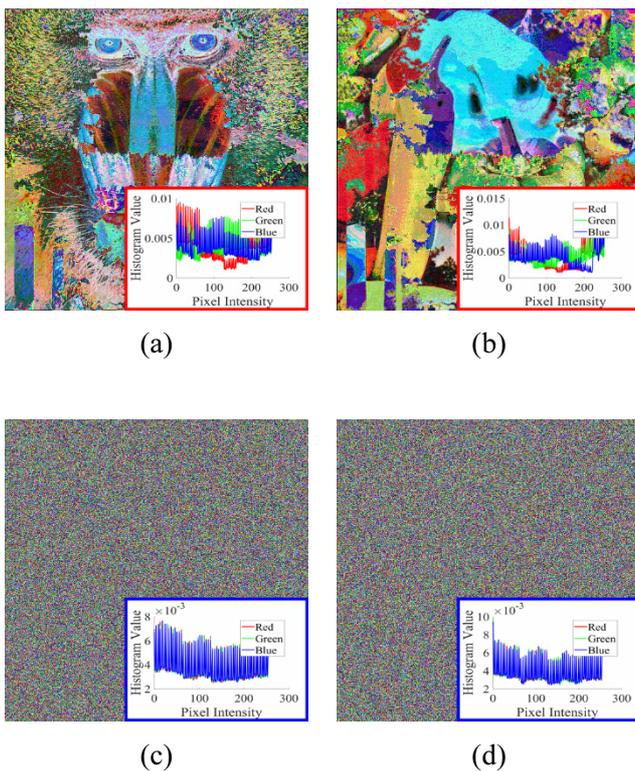
**Figure 10.** The results of (a, c)  $S_1 \oplus S_2$  and (b, d)  $S_2 \oplus S_3$ . Images in (a)-(b) and (c)-(d) are from [7] and the proposed method with double masking coefficients, respectively.
