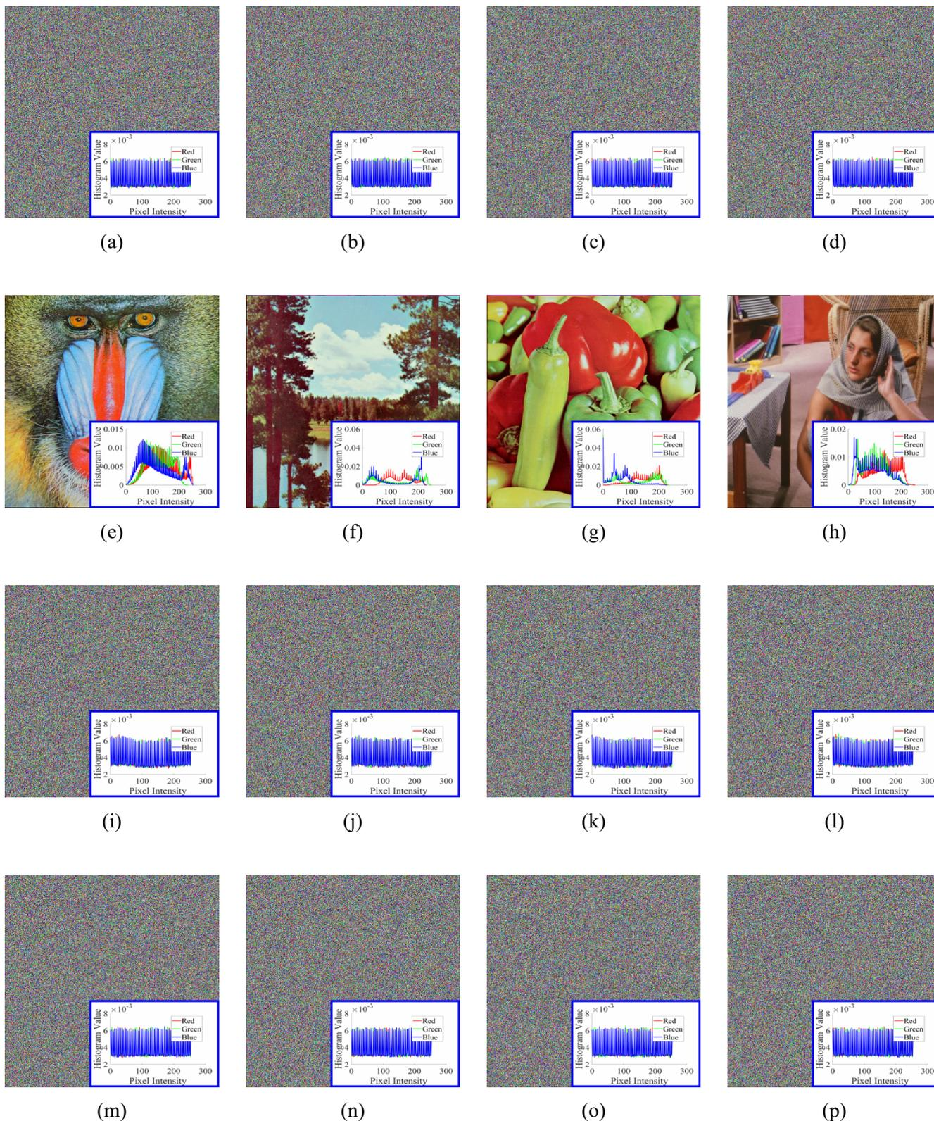
**Figure 8.** Proposed method with double masking coefficients, for  $n = 4$ : (a)-(d)  $\{S_1, S_2, S_3, S_4\}$ . (e)-(h)  $\{\tilde{I}_1, \tilde{I}_2, \tilde{I}_3, \tilde{I}_4\}$  recovered with correct chaotic keys. (i)-(l)  $\{\tilde{I}_1, \tilde{I}_2, \tilde{I}_3, \tilde{I}_4\}$  recovered with incorrect chaotic keys. (m)-(n)  $\{\tilde{I}_1, \tilde{I}_2\}$  recovered from  $n-1$  shared images. (o)-(p)  $\tilde{I}_1$  recovered from  $n-2$  and  $n-3$  shared images, respectively.
