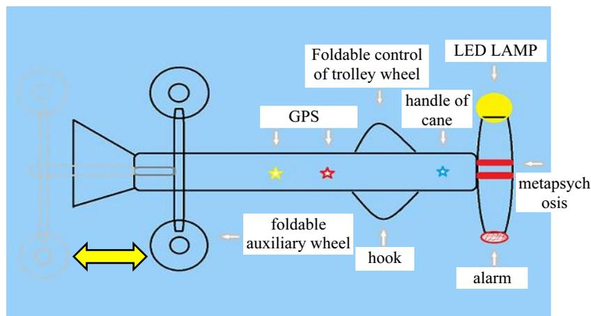
**Figure 2.** IoT smart cane design
