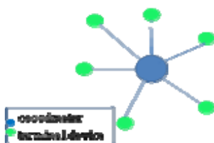
Figure 1. Star topology of Zigbee
