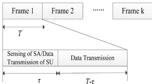
**Figure 3.** Frame structure of proposed spectrum-sensing framework
