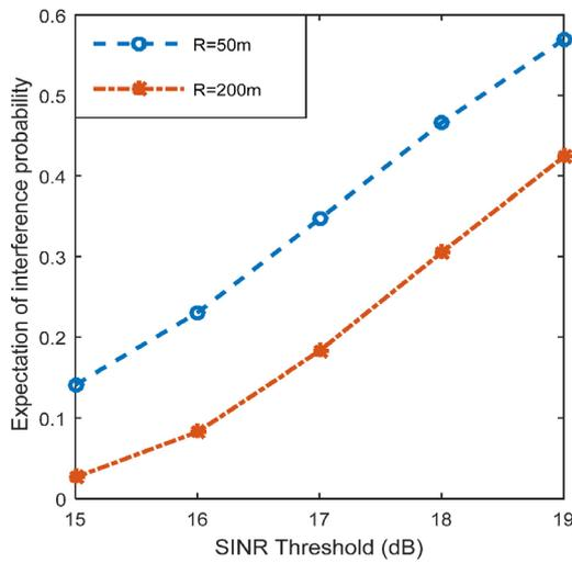
**Figure 10.** Expected interference probability versus various SINR thresholds
