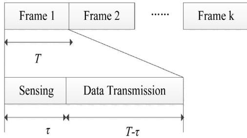
**Figure 2.** Frame structure of a conventional CR system
