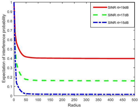
**Figure 9.** Variation of expected interference probability versus different network coverage ratio
