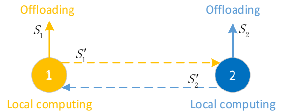
Figure 2. MT1 forward some data via short link to the neighbor/header node then the header performs some simple computation locally then offloads the data to the server.
