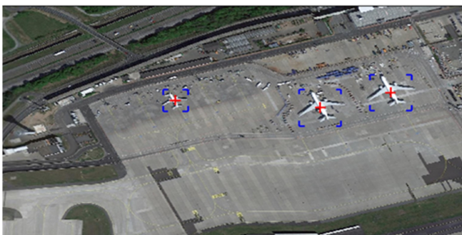
Figure 14. The recognition result of plane target-2
