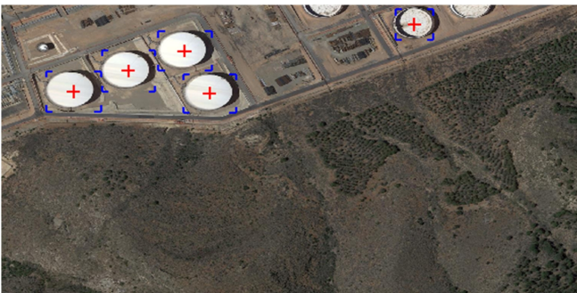
Figure 12. The recognition result of oil tank target-2
