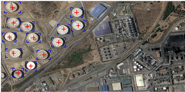
Figure 11. The recognition result of oil tank target-1
