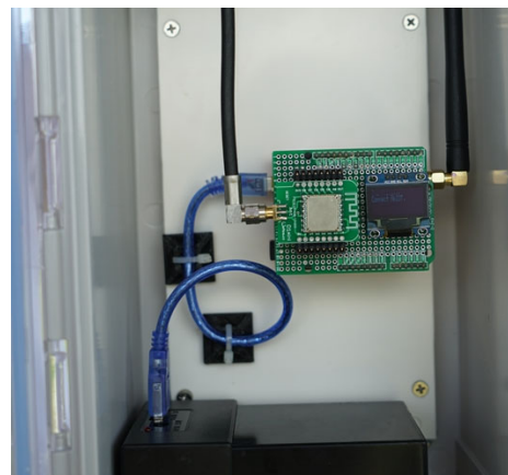
Figure 6. All electronic devices are put in a waterproof control box
