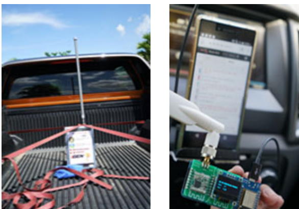
Figure 9. The LoRa node with the GPS was place in the vehicle for testing the distance of the communication
