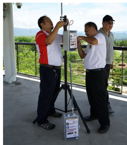
Figure 7. The low cost single private LoRa gateway connecting with the public AIS NB-IOT with the stand and the Omni antenna
