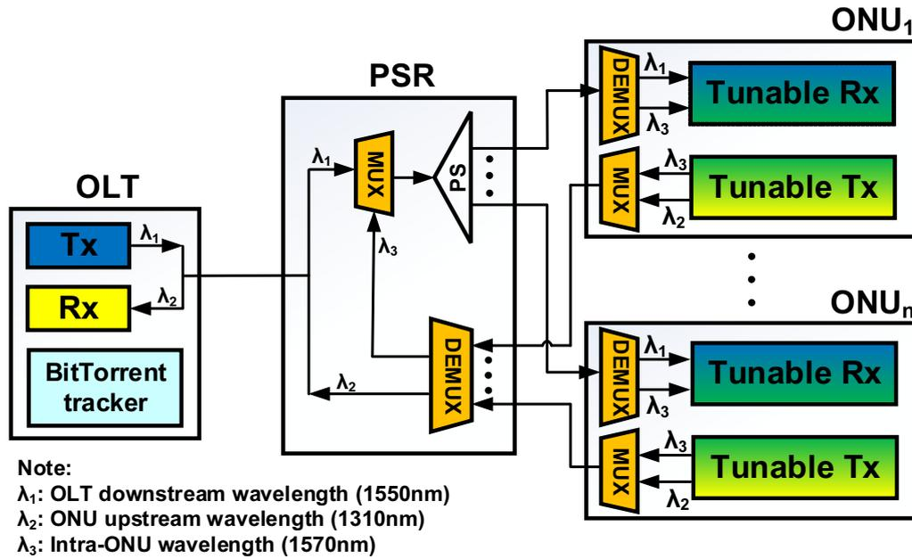
Figure 1. Proposed BitTorrent locality-aware process in the EPON system architecture
