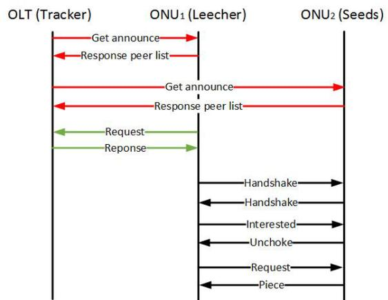
Figure 3. BT operation in the EPON
