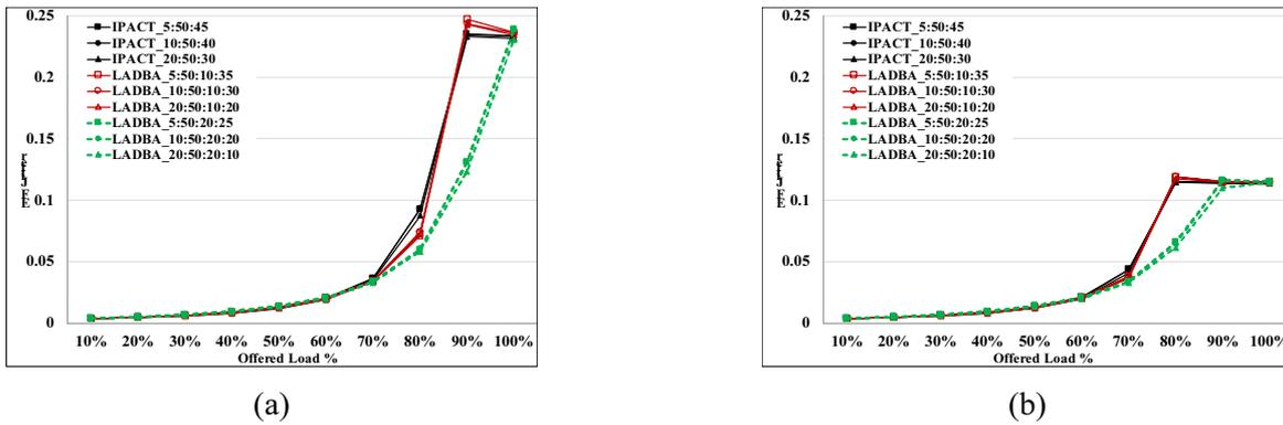
Figure 6. Jitter with cycle times of: (a) 1.5 ms and (b) 1.0 ms
