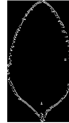
Figure 20. The result of blob detection from horizontal edge enhancement of a holy basil leaf
