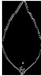
Figure 28. The result of blob detection from horizontal edge enhancement of a sweet basil leaf
