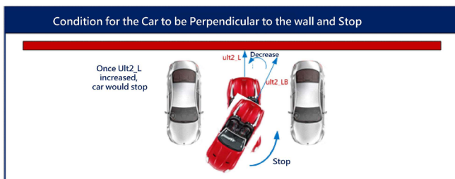
Figure 17. Condition for the car to be perpendicular to the wall and stop
