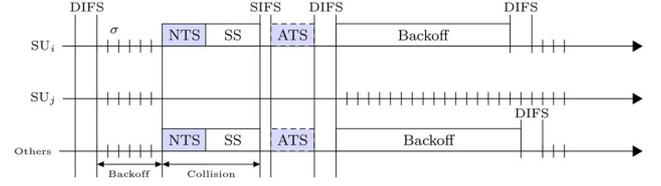
(b) Collision of multiple NTS packets
