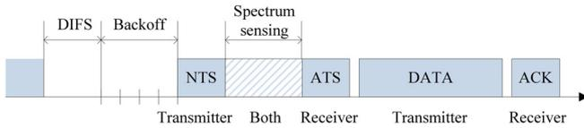
**Figure 1.** Typical packet transmission procedure
