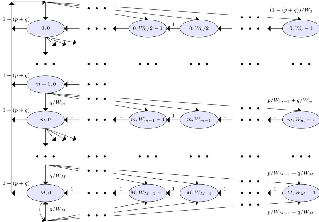
Figure 4. Markov chain model of the backoff process
