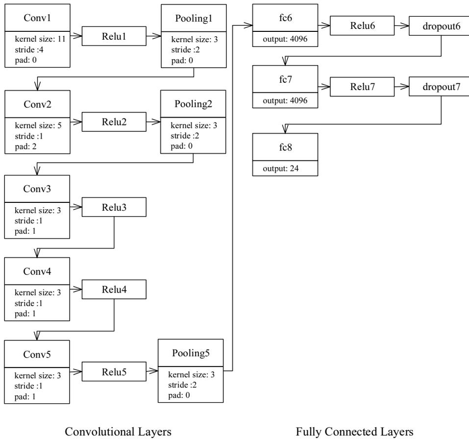
**Figure 4.** The improved Architecture of CaffeNet The output number of the last fully connected layer is modified to 24. The left part are 5 convolutional layers with regular layers and pooling layers. The right part are 3 fully connected layers with regular layers and drop out layers
