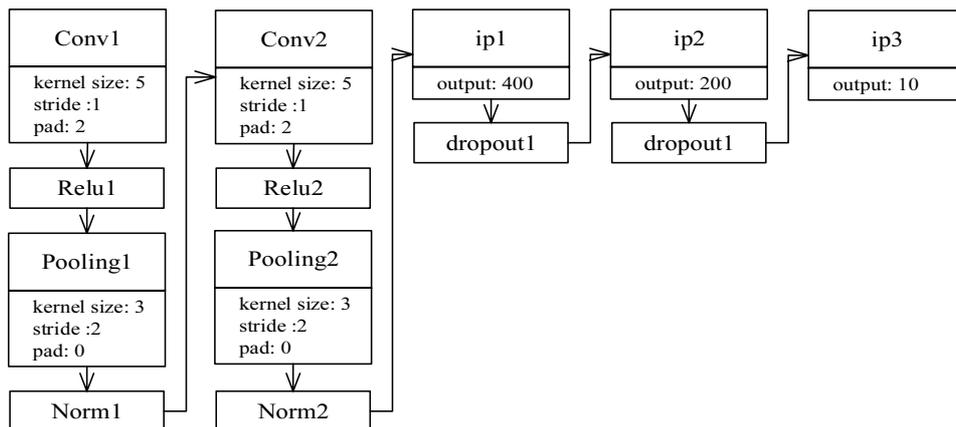
**Figure 3.** The network architecture of CNNs for training models on CIFAR-10 data set and the small-scale data set
