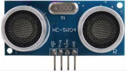
Figure 3. The ultrasonic transmitter and receiver used for measuring distance
