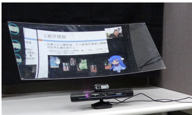
Figure 3. Image of the affective learning system (combined with motion-sensing, augmented reality, and mid-air projection technologies)
