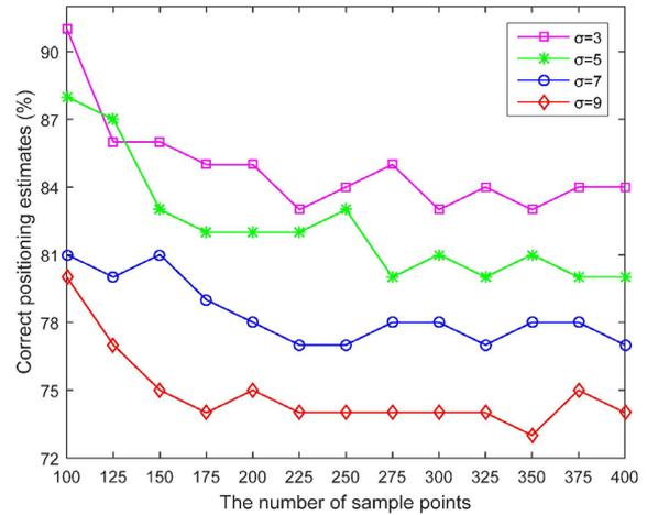
Figure 17. Percentage of correct positioning estimates obtained using fuzzy rectangular zone splitting method
