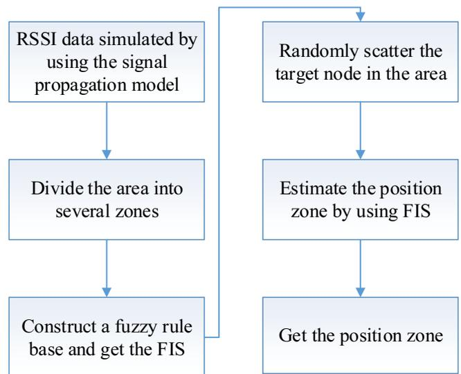
Figure 3. Processing flow of proposed system
