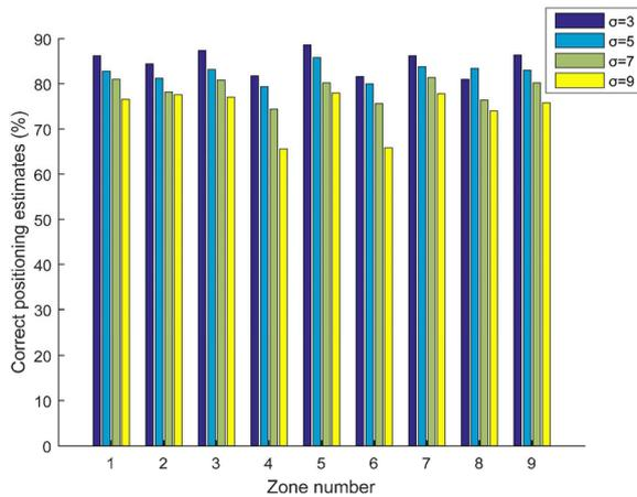
**Figure 21.** Positioning performance of fuzzy rectangular splitting method in nine specific zones
