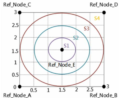
Figure 7. RSSI power level from reference node E [13]
