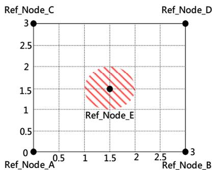
Figure 19. Area of central reference node (radius of 0.5 m)
