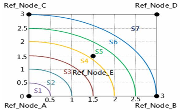
Figure 6. RSSI power level from reference node A [13]
