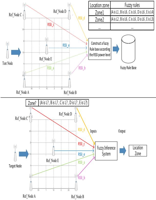
Figure 4. FIS structure of proposed zone-based positioning system
