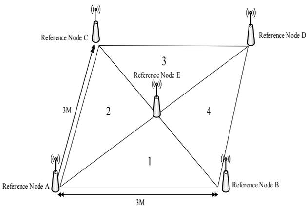
Figure 8. Triangular splitting method [13]
