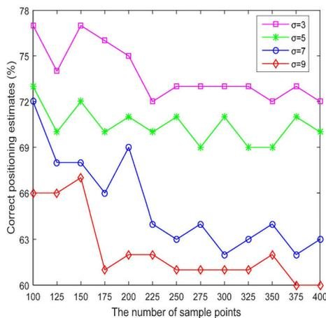
Figure 16. Percentage of correct positioning estimates obtained using fuzzy triangular splitting method
