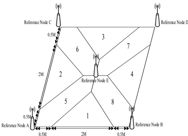
Figure 9. Fuzzy triangular splitting method [13]
