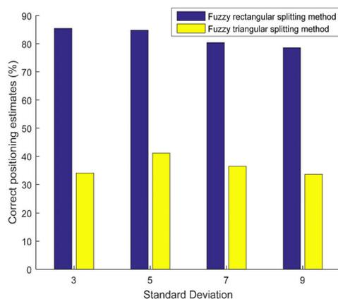
Figure 20. Positioning performance of two fuzzy zone splitting methods in region of central reference node
