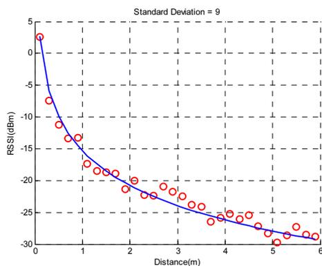
Figure 14. Signal propagation model with  $\sigma=9$
