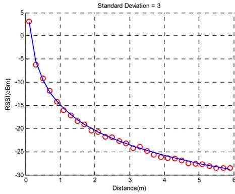
Figure 11. Signal propagation model with  $\sigma=3$
