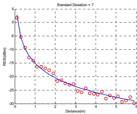
Figure 13. Signal propagation model with  $\sigma=7$
