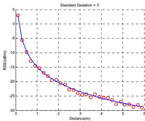
Figure 12. Signal propagation model with  $\sigma=5$
