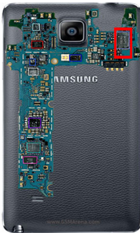
Figure 1. Bluetooth antenna in Samsung Galaxy Note 4
