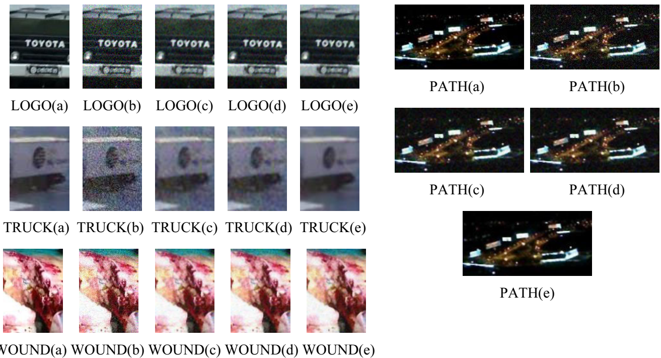
Figure 4. The visual comparison of filtering results obtained by the three denoising methods, (a) is the original color image, (b) is a color image added noise with \sigma = 45 , (c) is the filtering result of PR, (d) is the filtering result of CNLM, (e) is the filtering result of our method
